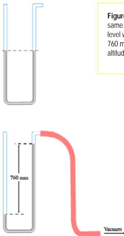
**Figure 2.** (Left, above) If mercury any fluid is placed in an open U-tube its level will be the same on both sides. (Left, below) If a vacuum is drawn on one side, the mercury will rise to the level where the mass of the liquid is balanced by the pressure of the atmosphere. That rise is 760 mm under the Earth's atmosphere. Of course, the atmospheric pressure varies with your altitude and changes slightly over time. 760 torr is "normal" atmospheric pressure at sea level.
